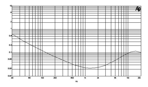
Most of the distortion in the M2 represents the performance of the auto-former which performs the voltage amplification. Many magnetic circuit products were evaluated in the development of this amplifier – some measured better, some measured worse. The final choice went to the part that actually sounded the best in blind listening sessions.
