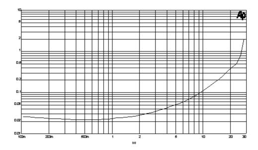
Here is that distortion curve into 4 ohms:
