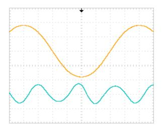
1.7% harmonic distortion waveform at 20 watts, 500 Hz, 8 ohms, w/o feedback
