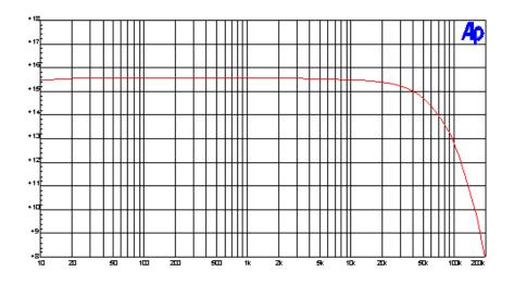
Frequency response of the amplifier, -3 dB down just above 100 Khz
