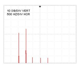
0.04% harmonic distortion spectrum at 500 Hz, 1 watt, 4 ohms, w/o feedback
