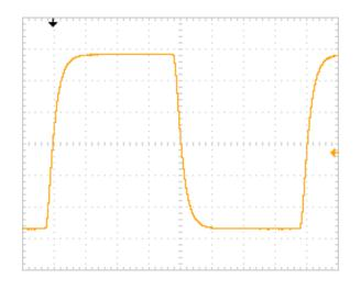
50 Khz square wave at 2 watts into 4 ohms.
