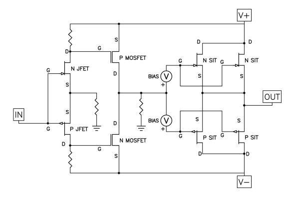
If you have absorbed the contents of the previous articles, you probably have a good picture of what is going on. To make it a little easier, I have identified the generic part types, and also the pin names: Drain, Source and Gate. You can see the input and output points, and also the two voltage sources used create the DC Gate voltages that set the output transistors to the desired bias current.
