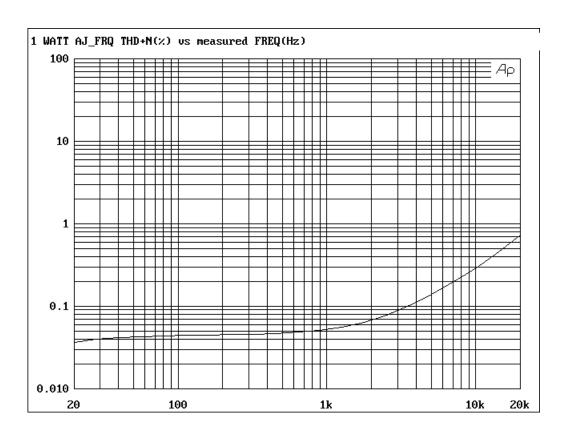
**DISTORTION VS FREQUENCY @ 1 WATT**
